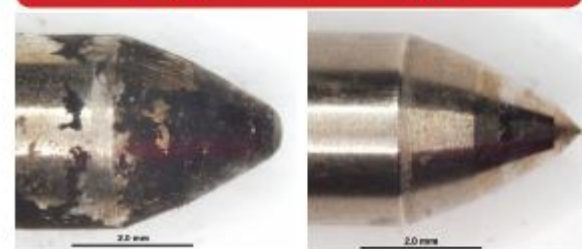
High Pressure Common Rail injectors before and after clean-up with fuel treated with Diesel Kleen +Cetane Boost.
