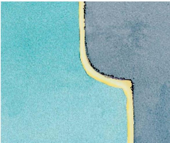
**The protective layer created by Fleetguard DCA prevents the aluminum from corroding.**
