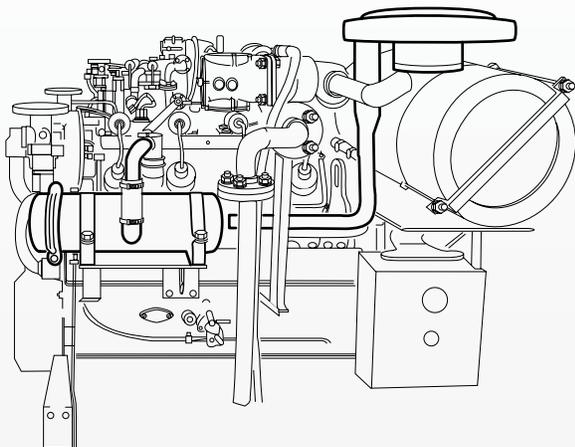
These filters were originally developed to prevent oily crankcase fumes from fouling the intake air filters and coating the engine room walls, but now offer many other advantages.
