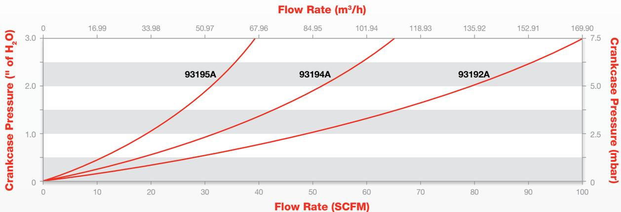
Sizing and installation of the EcoVent Recirculator require an initial maximum pressure of 0" to 0.3" H<sub>2</sub>O (0-0.75 mbar) at engine load with a clean element.
