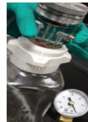
Figure 11. Using the vacuum release valve
