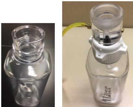
Figure 2. Connecting the filter holder
