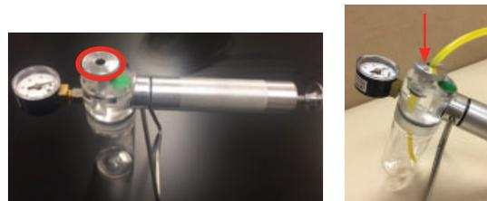
Figure 6. Inserting the Tygon® fuel tubing
