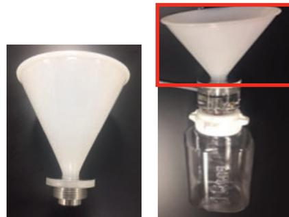
Figure 5. Connecting the funnel assembly
