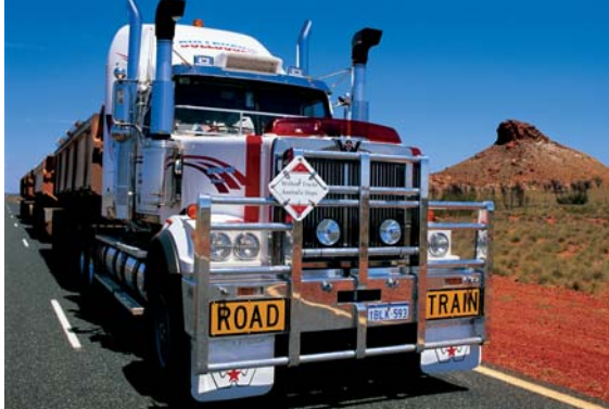
Australia Road Train with Cummins ISM carrying 120,000 lb load
