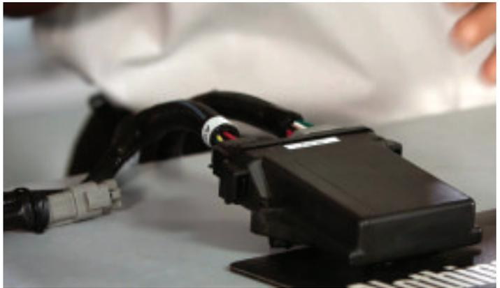
The FleetguardFIT system from Cummins Filtration incorporates intelligent sensors (above, top right) that are added to the air, fuel and lube filter assemblies and connect to a stand-alone control module to provide real-time monitoring of the filters. The system is designed for on- and off-highway vehicles and equipment, as well as stationary and marine applications.
